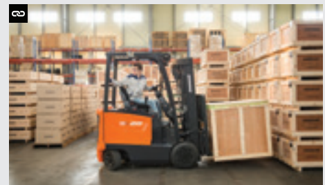
BC25S-7: 2.5 ton electric forklift
